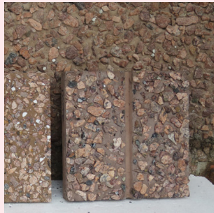
Hanasaari models 2015. For the renewed concrete panels. The colored concrete mass was still in production by Bayer and the red stone came from the original quarry in Kemiö. Photo: Architects Kirsi Korhonen and Mika Penttinen.
